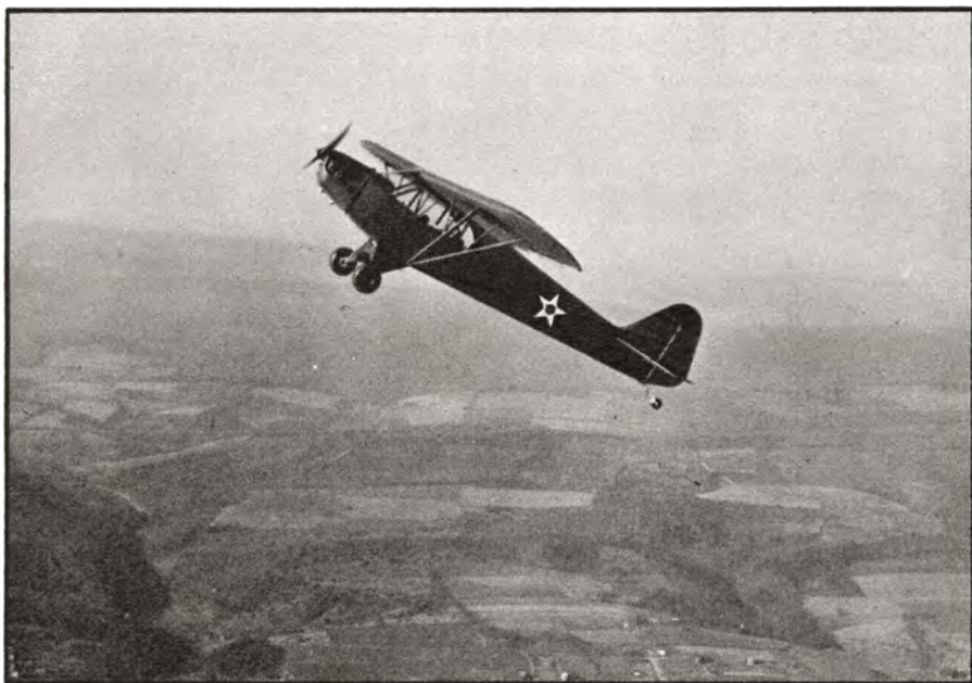
THE FIRST TEST Alma gives the O-59 a climb, to determine the engine's ability to "rev up" (speed) without overheating—important because "jeeps" take off over obstacles from small fields. She averages 25 tests a week, depending on weather.
